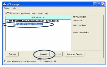
3. The following message is displayed to warn you that you have to follow the installation instructions in the manual of the MFP. If the MFP is requiring you to connect the MFP to your computer directly, please click "Connect".
